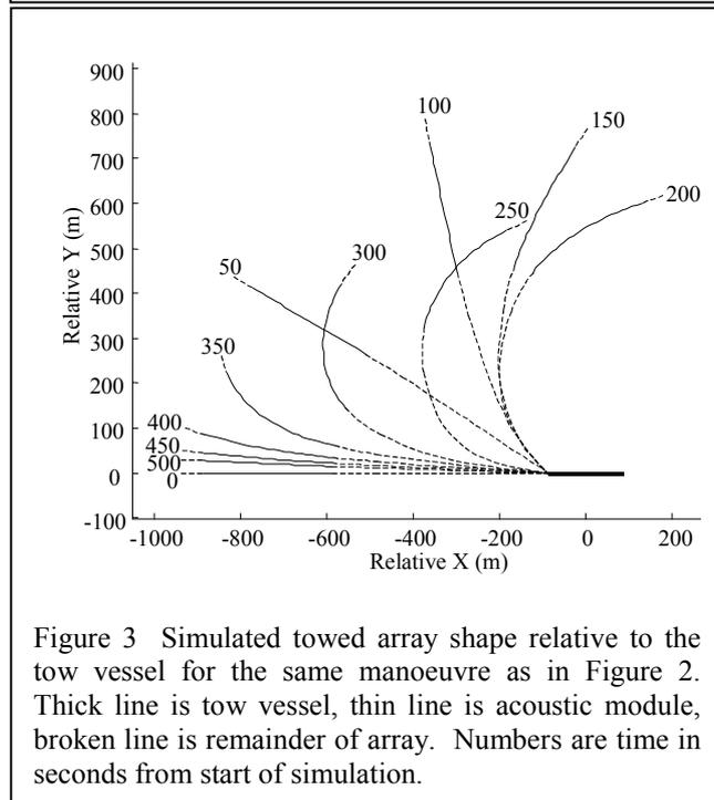
Figure 3 Simulated towed array shape relative to the tow vessel for the same manoeuvre as in Figure 2. Thick line is tow vessel, thin line is acoustic module, broken line is remainder of array. Numbers are time in seconds from start of simulation.
