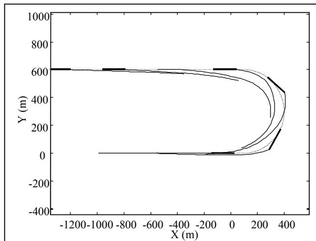
Figure 2 Six snap-shots of the simulated towed array shape during a U-turn manoeuvre. Thick line is vessel, dotted line is vessel track, thin line is towed array. Simulation starts with vessel at (0, 0) and moving to the right. Vessel speed = 5 m/s, turn radius = 300 m, tow cable length = 400 m.
