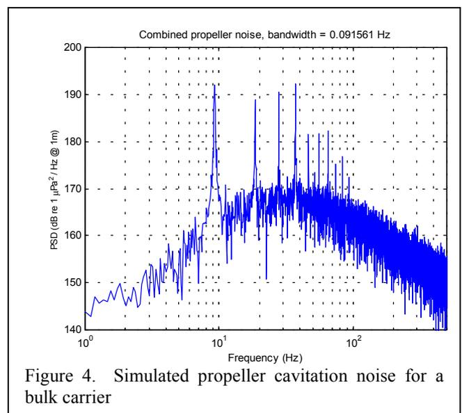
Figure 4. Simulated propeller cavitation noise for a bulk carrier
