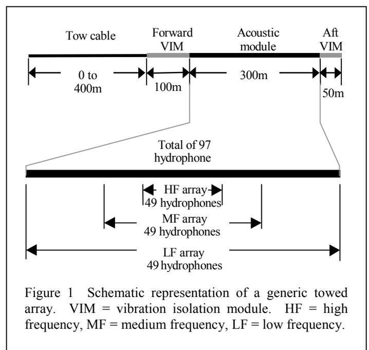
Figure 1 Schematic representation of a generic towed array. VIM = vibration isolation module. HF = high frequency, MF = medium frequency, LF = low frequency.
