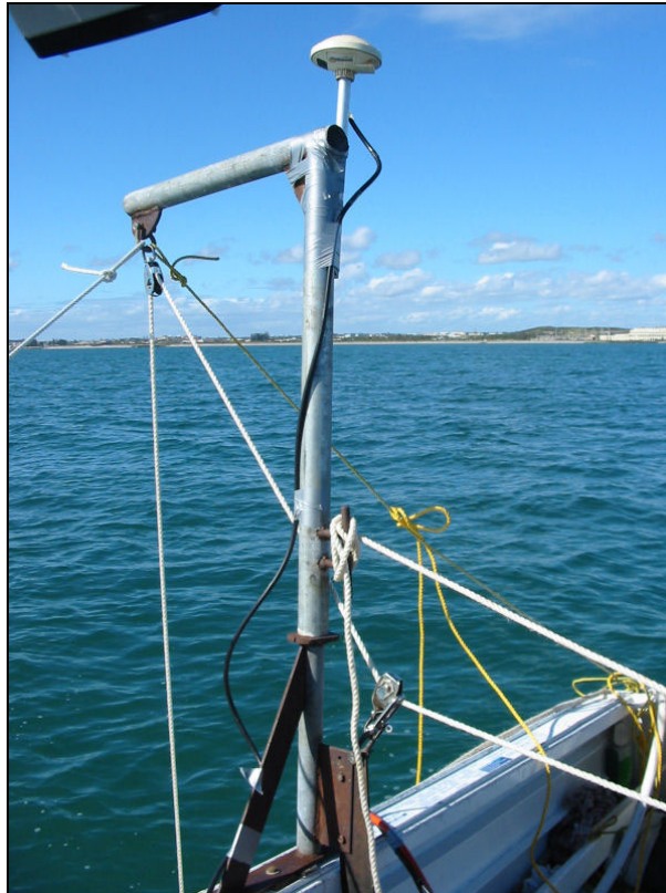
Figure 5: Davit fitted to boat as used for ESP wet-end deployment (GPS antenna visible on top of davit)
