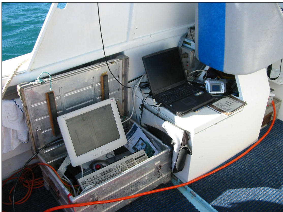
Figure 7: The setup of some of the ESP equipment on the back deck of “Jabiru”. (EQ60 computer (left), laptop computer running “ESPañolito”, video camera, Omnistar GPS, and various power supplies).
