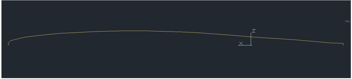
Figure 19: Top view of the half teardrop produced from the data points of y-displacement delta modelled in AutoCAD.
