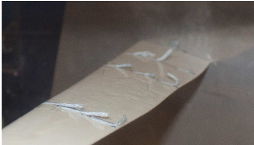
Figure 25: Separated tell tale behaviour. (Cropped from photo #8369)
