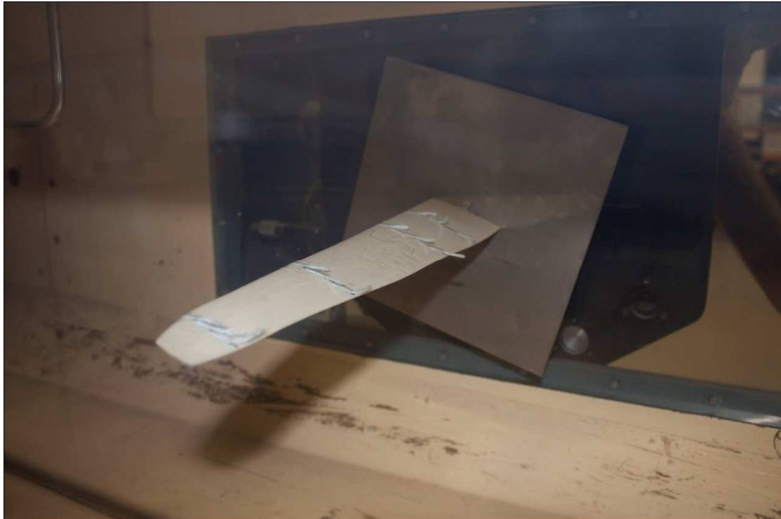
Figure 38: Fin model oriented at 16^\circ to the flow, with wind speed of 14.6 \text{ ms}^{-1} . (Photo #8338)
