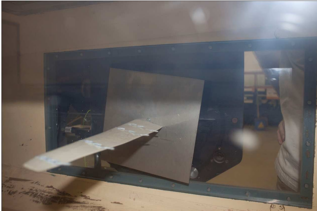
Figure 39: Fin model oriented at 8^\circ to the flow, with wind speed of 20.9 \text{ ms}^{-1} . (Photo #8361)
