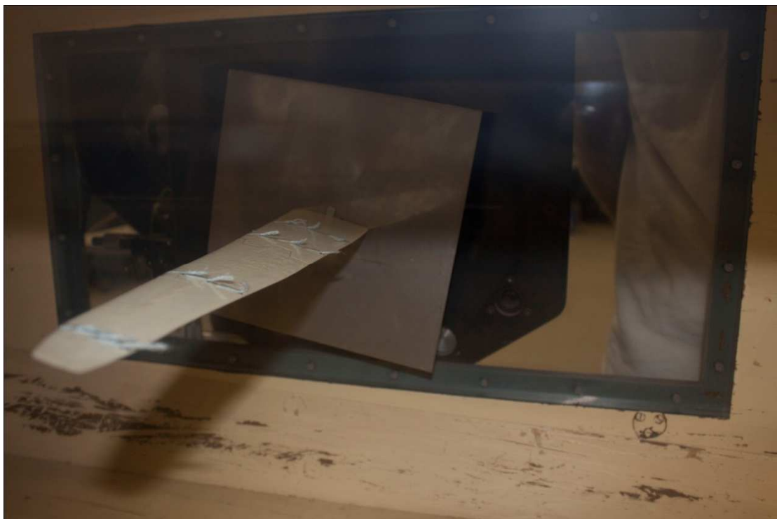
Figure 40: Fin model oriented at 10^\circ to the flow, with wind speed of 20.9 \text{ ms}^{-1} . (Photo #8352)
