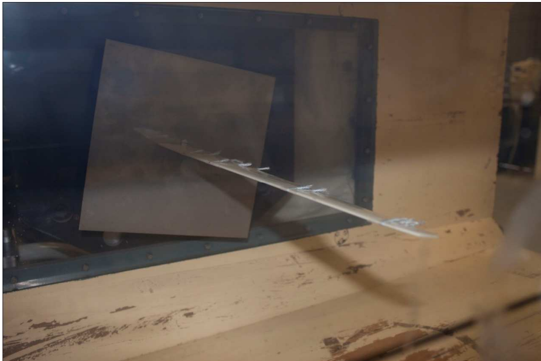
Figure 36: Fin model oriented at 12^\circ to the flow, with wind speed of 14.6 \text{ ms}^{-1} . (Photo #8318)
