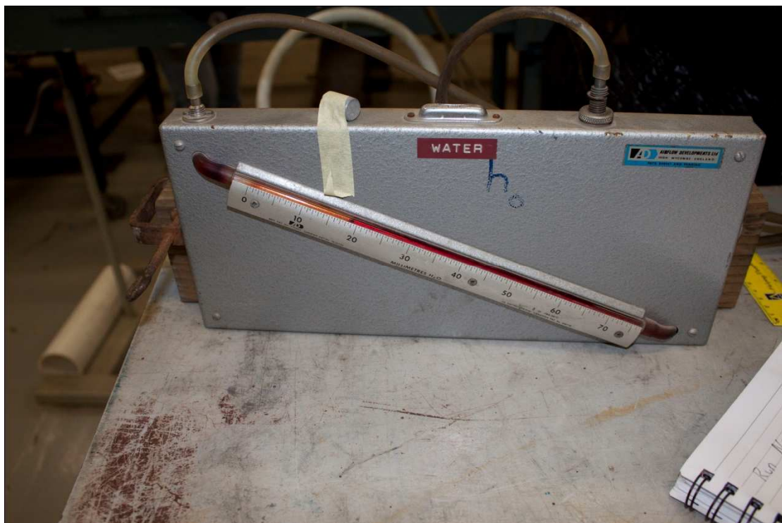
Figure 34: Manometer used to show the pressure difference measured by the Pitot tube.
