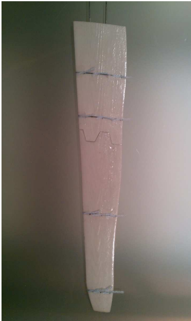
Figure 30: Model fin with tell tales attached at 10%, 50%, and 90% of the chord of model y-displacements bravo, charlie, echo and golf. (IMAG0146)
