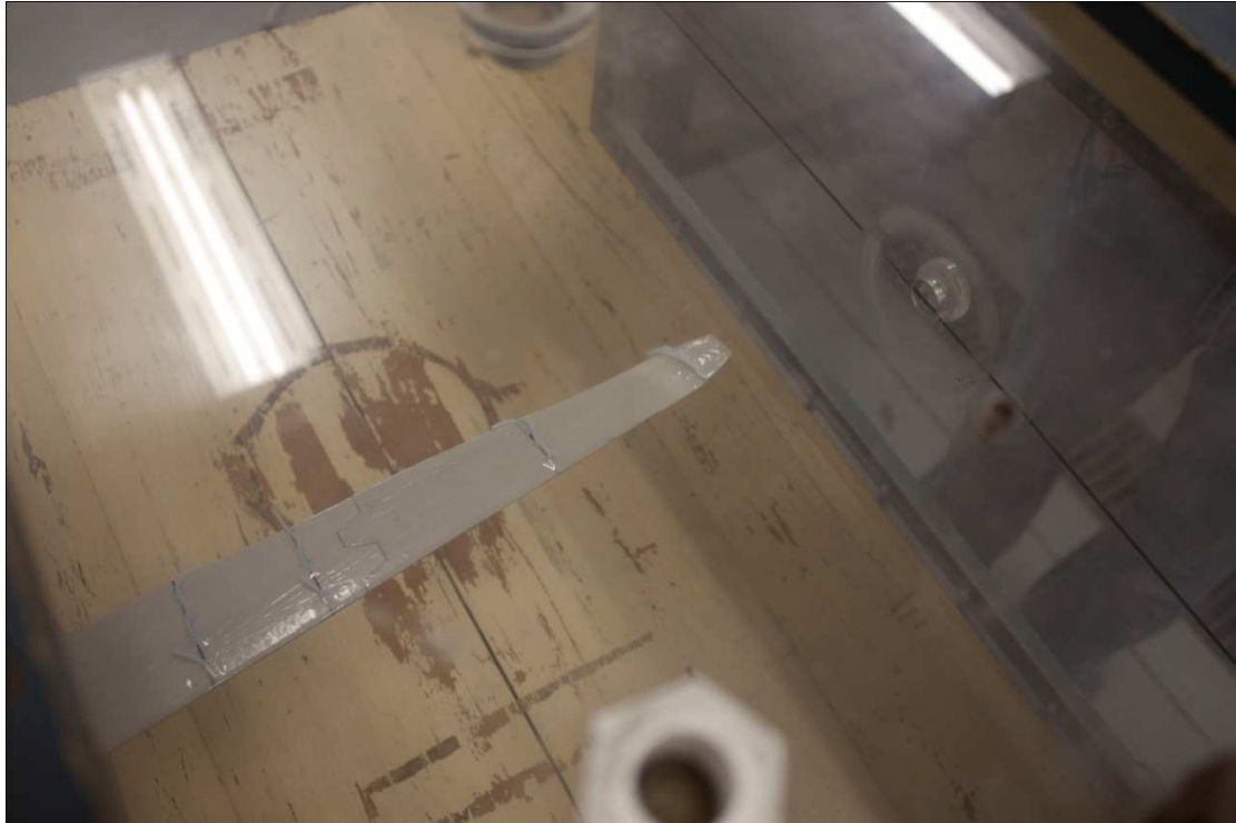
Figure 37: Fin model oriented at 14^\circ to the flow, with wind speed of 14.6 \text{ ms}^{-1} . (Photo #8321)
