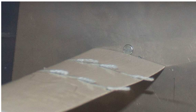
Figure 24: Attached tell tale behaviour. (Cropped from photo #8361)
