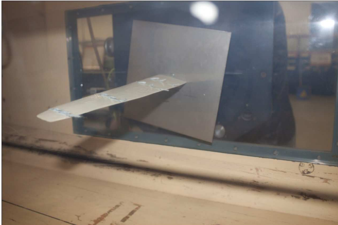
Figure 35: Fin model oriented at 10^\circ to the flow, with wind speed of 14.6 \text{ ms}^{-1} . (Photo #8313)
