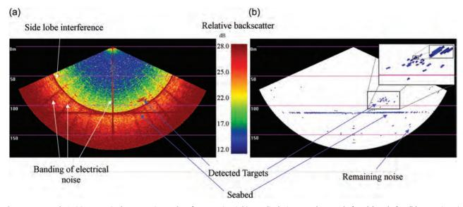
**Figure 2.** Example RESON 7125 Seabat acoustic swathe of aggregating S. *hippos* displaying an echogram before (a) and after (b) acoustic noise removal. Volume backscatter values were thresholded at 12 and 28 dB, graduated as per the colour bar. Coherent electrical noise, side-lobe noise ("spoking"), together with detected targets and seabed are highlighted. Insets show expansions of detected targets highlighting one target comprising a cluster of several samples (top right).
