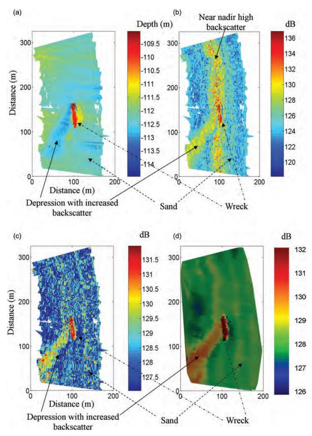
**Figure 5.** Bathymetry (a), uncorrected backscatter (b), corrected backscatter (c), and smoothed backscatter (d) acquired from a single acoustic transect of the Outer Patch site. Axes display relative distance in metres, while depth and relative backscatter are shown as per the respective colour bars.
