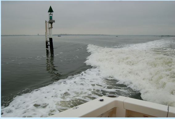
Wake produced by a recreational vessel, being measured by CMST's pressure sensor waverecorder mounted on Quarry Point pylon, Perth.
