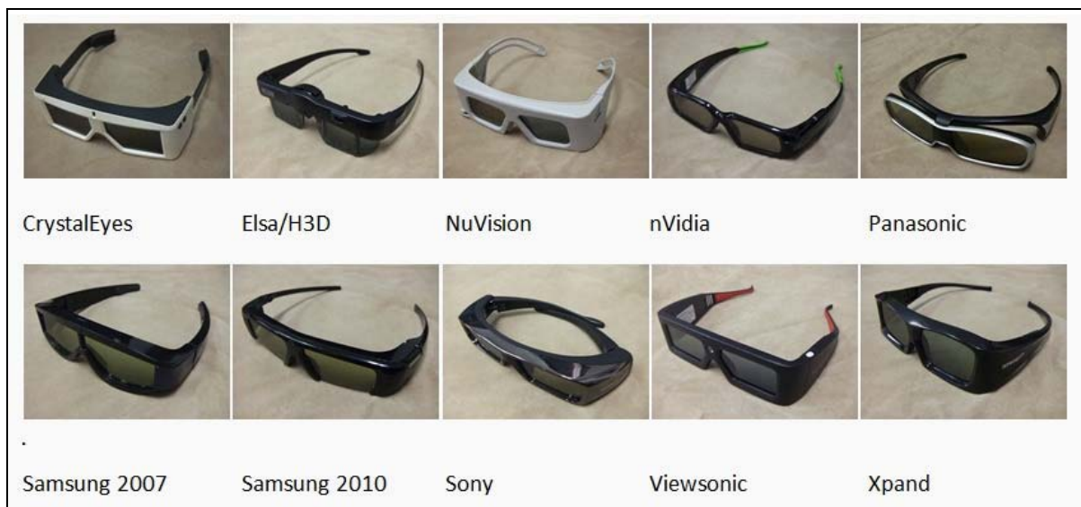
Figure 1: The ten active shutter glasses tested in this study: (a) StereoGraphics Crystaleyes CE-1, (b) ELSA/H3D, (c) NuVision 60GX, (d) NVIDIA 3D Vision, (e) Panasonic TY-EW3D10U, (f) Samsung 2007, (g) Samsung (2010) SSG-2100AB, (h) Sony TDG-BR100, (i) Viewsonic PGD-150 DLP Link, (j) Xpand X103 Universal.
