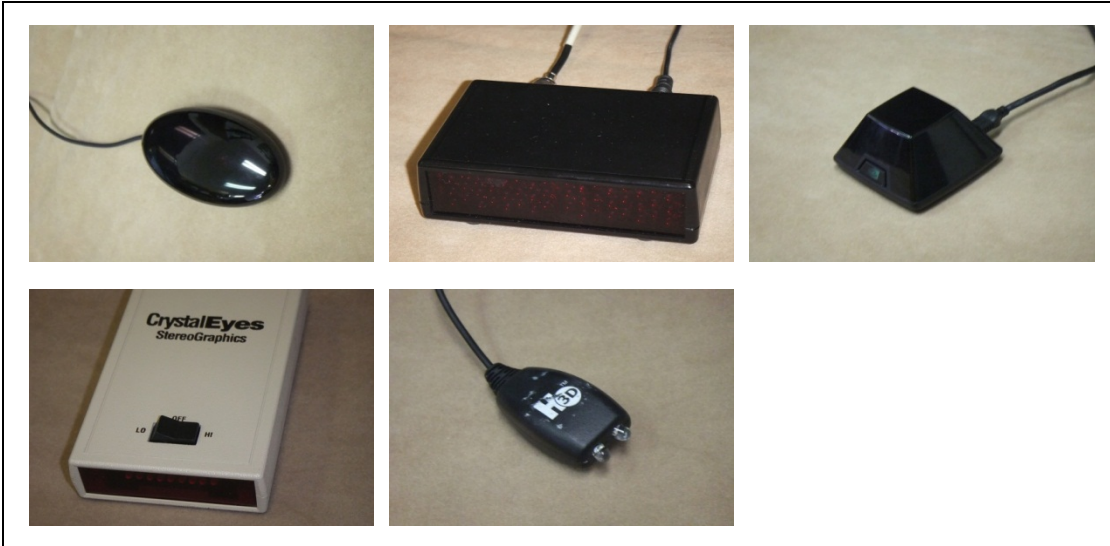
Figure 2: Some of the stand-alone IR 3D emitters tested: (a) Samsung 2007, (b) NuVision, (c) NVIDIA, (d) CrystalEyes 1, and (e) H3D/ELSA.
