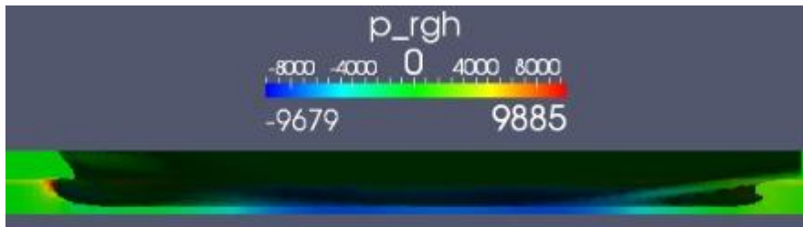
Figure 6.7: Dynamic pressure of ship and channel OpenFOAM, T=13.0m , U=10kn
