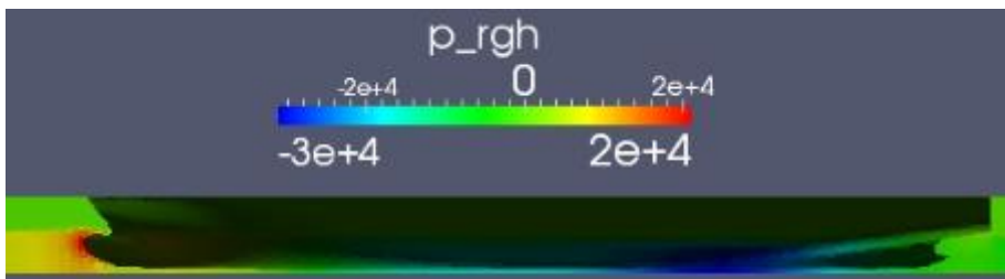
Figure 6.8: Dynamic pressure of ship and channel OpenFOAM, T=14.5m , U=14kn
