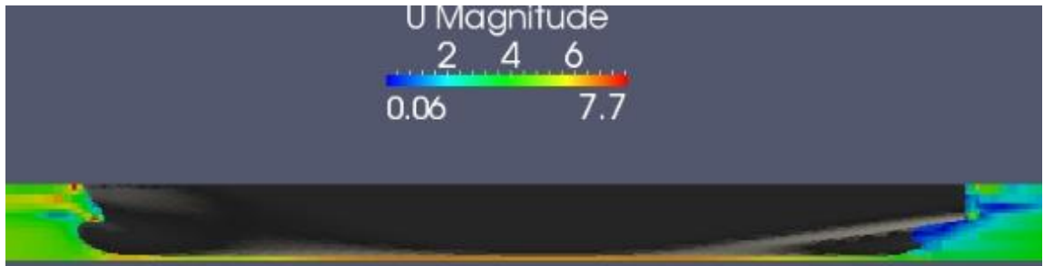
Figure 6.10: Channel fluid velocity (m/s) OpenFOAM, T=14.5m , U=10kn
