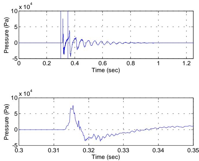
Figure 3. Near-field hydrophone signal and expanded signal
