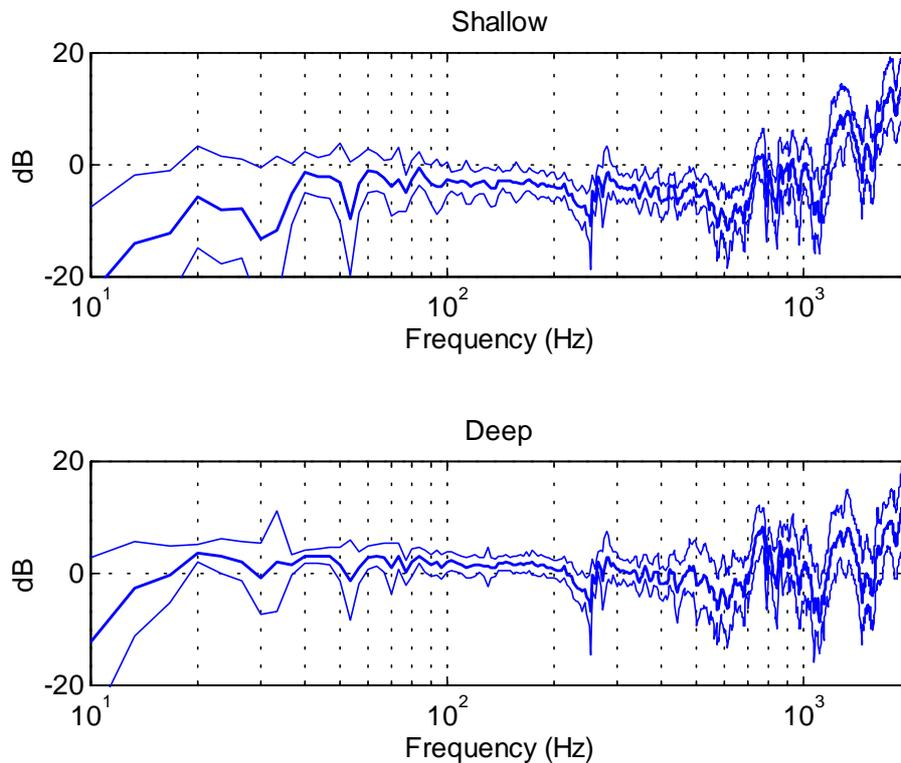
Figure 6. Thick line is mean of the dB differences between the predicted and measured signals as a function of frequency for 42 shots at ranges varying from 80 m to 1000 m. Thin lines are mean  $\pm$  1 standard deviation. Top plot is for shallow hydrophone, bottom plot is for deep hydrophone.
