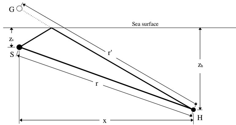
Figure 2. Geometry for calculation of received signal due to direct path and surface reflection. S is the source, G is the ghost or image source caused by reflection at the sea surface and H is the receiving hydrophone.
