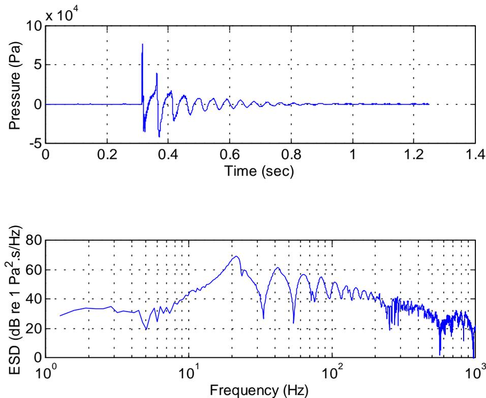
Fig 1. Typical signal from an air-gun and its energy density spectrum
