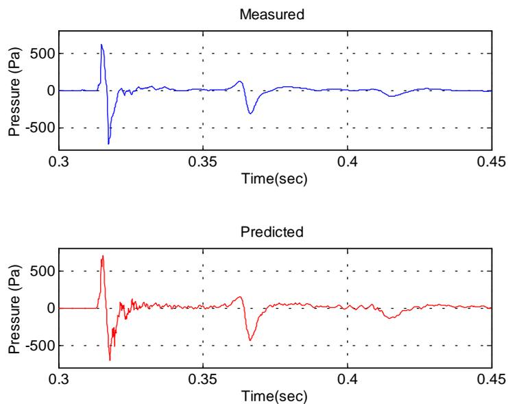
Figure 4. Time domain comparison of predicted and measured signals for a shot at 107 m range, a gun depth of 3.6 m, and a hydrophone depth of 46 m.
