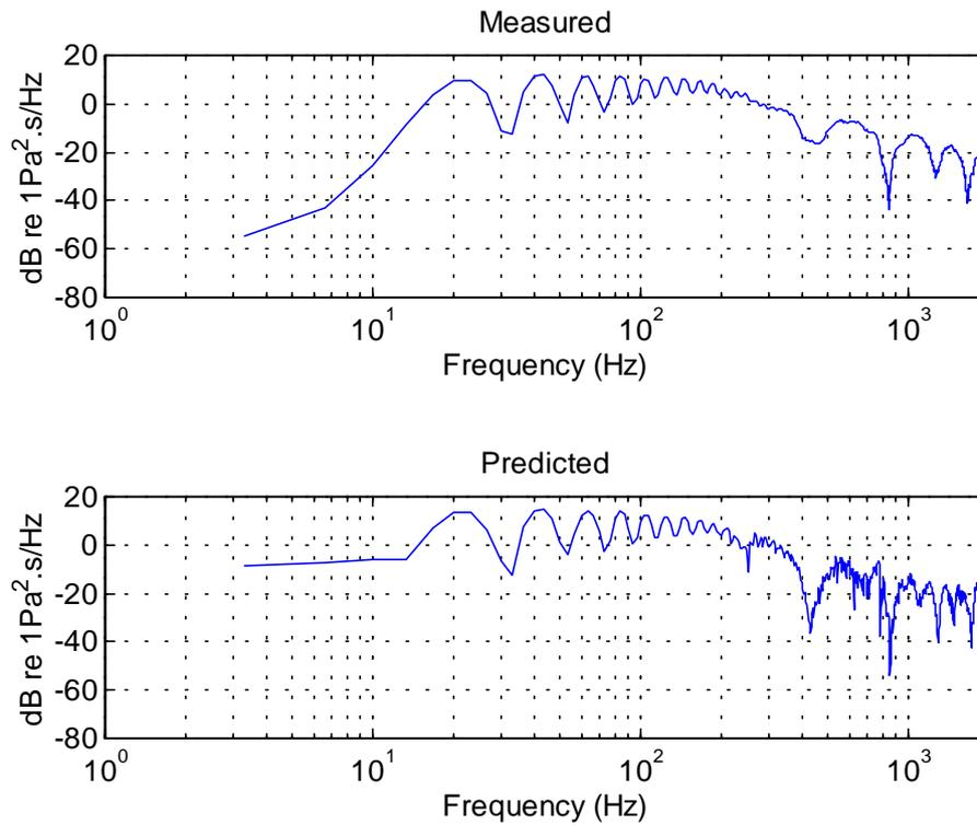
Figure 5. Frequency domain comparison of predicted and measured signals for a shot at 107 m range, a gun depth of 3.6 m, and a hydrophone depth of 46 m.
