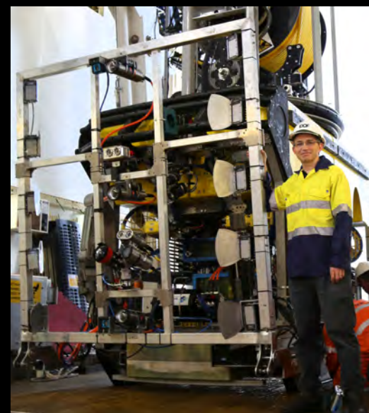
DOF Subsea ROV with custom lighting and camera frame attached. Photo: Joshua Hollick
