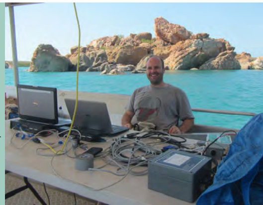
CMST's Iain Parnum running the Odom ES3 multi-beam echo-sounder in the Kimberley.
