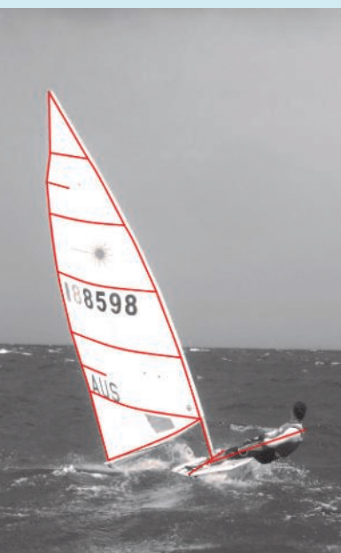
Image of sail analysed using CMST SailTool software, taken during dinghy trialling off Fremantle Sailing Club.
