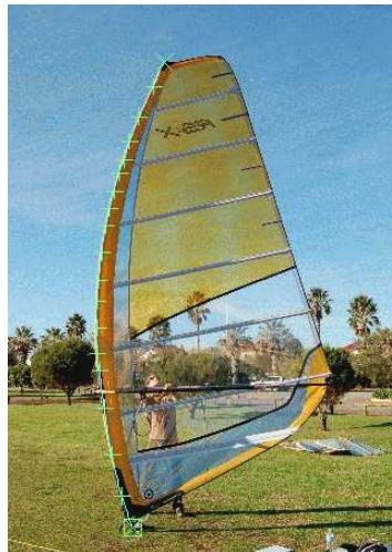
Figure 2: Digitized SailTool image of fore-aft mast bend
