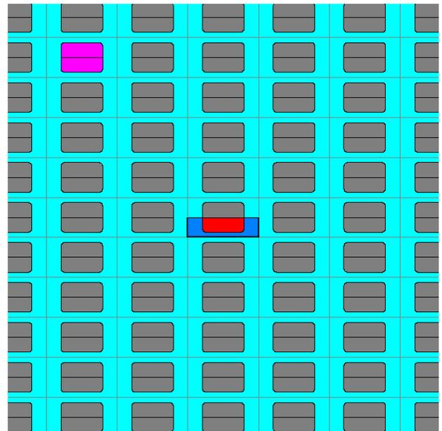
**Figure 13. Image system stretching to infinity for ship in a shallow rectangular canal (stern view). Submerged hull shown in red. Image hulls shown in grey. Example image hull shown in pink as used in Figure 15.**
