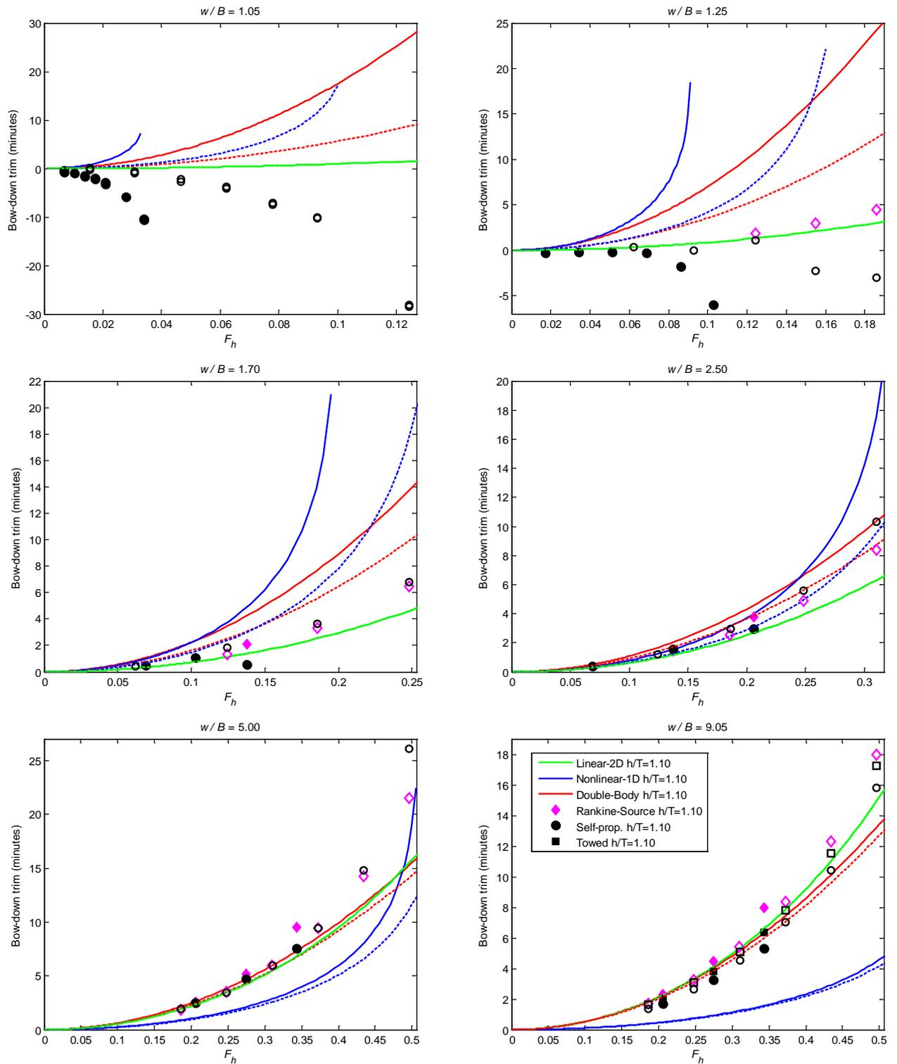
**Figure B1.** Dynamic trim predictions and model test results for KVLCC2 in rectangular canals of increasing  $w/B$  ratio. The same legend applies to all subplots. Dashed lines and unfilled markers are corresponding results for  $h/T=1.35$ . The *Linear-2D* results for both water depths are almost coincident.
