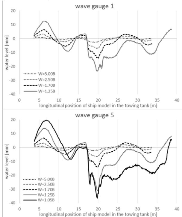
**Figure 4.** Wave registrations for two wave gauges at 5 different cross section widths
