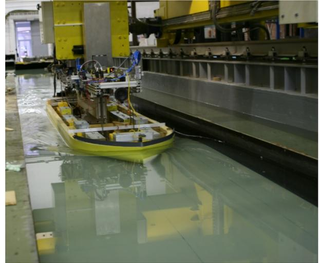
**Figure 2. KVLCC2 model during an experiment.**
