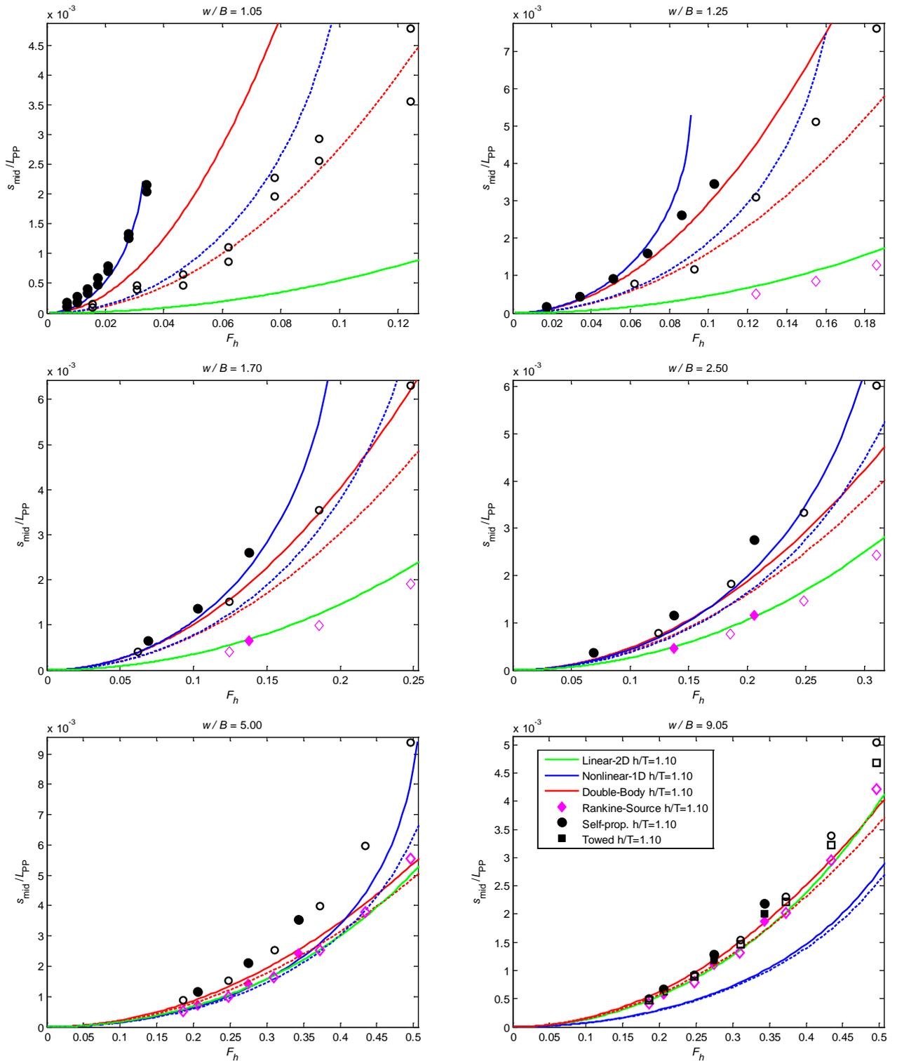
Figure A1. Midship sinkage predictions and model test results for KVLCC2 in rectangular canals of increasing  $w/B$  ratio. The same legend applies to all subplots. Dashed lines and unfilled markers are corresponding results for  $h/T=1.35$ . The *Linear-2D* results for both water depths are almost coincident.
