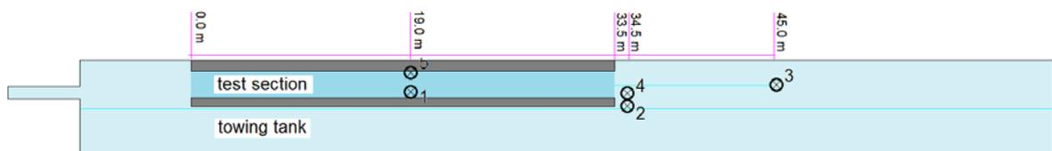
**Figure 3. Positions of the wave gauges in the towing tank**
