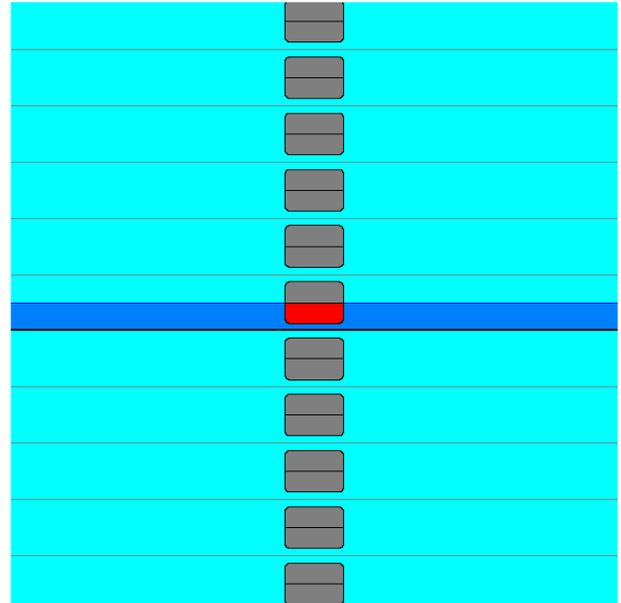
**Figure 12. Double-body method for a ship in shallow open water (stern view). Submerged hull shown in red, image hulls shown in grey.**
