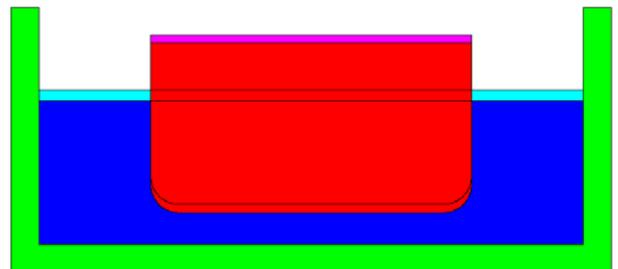
**Figure 10. *Nonlinear-1D* method. Pink shows static floating position, red shows squatted position. Light blue shows static free surface, dark blue shows actual free surface.**
