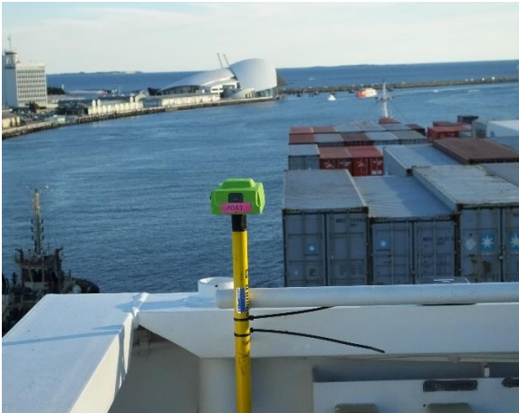
Figure 1. GNSS receivers setup. (a) Plan view of ship receivers. (b) Base station on pilot jetty in the CMA CGM LAMARTINE (outbound) transit. (c) Bow receiver in the MOL PARAMOUNT (outbound) transit. (d) Port receiver on bridge wing in the SAFMARINE MAKUTU (outbound) transit. (e) Starboard receiver on bridge wing in the SAFMARINE MAKUTU (outbound) transit.
