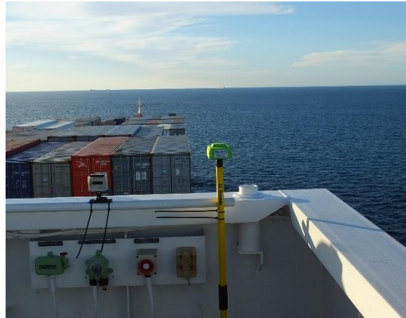
Figure 1. GNSS receivers setup. (a) Plan view of ship receivers. (b) Base station on pilot jetty in the CMA CGM LAMARTINE (outbound) transit. (c) Bow receiver in the MOL PARAMOUNT (outbound) transit. (d) Port receiver on bridge wing in the SAFMARINE MAKUTU (outbound) transit. (e) Starboard receiver on bridge wing in the SAFMARINE MAKUTU (outbound) transit.
